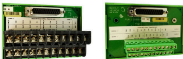
Figure 7: ET Blocks with screw terminals for lugged field wiring (left) and high-density “Euro” connectors for non-lugged field wiring (right)
